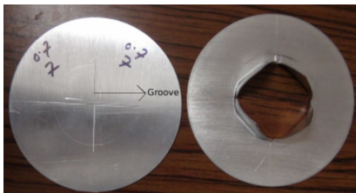
Figure 2.3: Aluminium diaphragm. Left: Before experiment. Right: After experiment.
