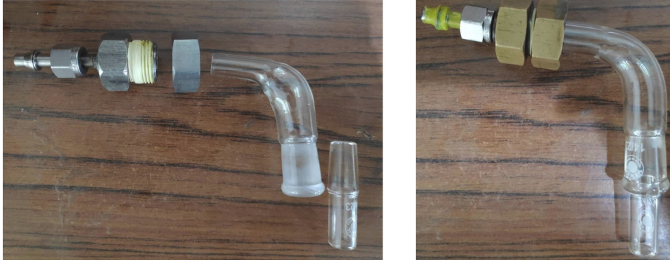
Figure 2.4: Sample loading adaptor. Left: assembled sample holder used to load sample into shock tube . Right: disassembled sample holder
