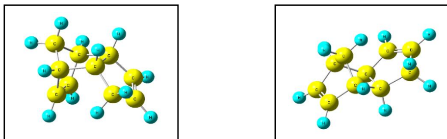
Figure 1.1. The molecular structure of DCPD (a) endo-DCPD (left) (b) exo-DCPD (right)
