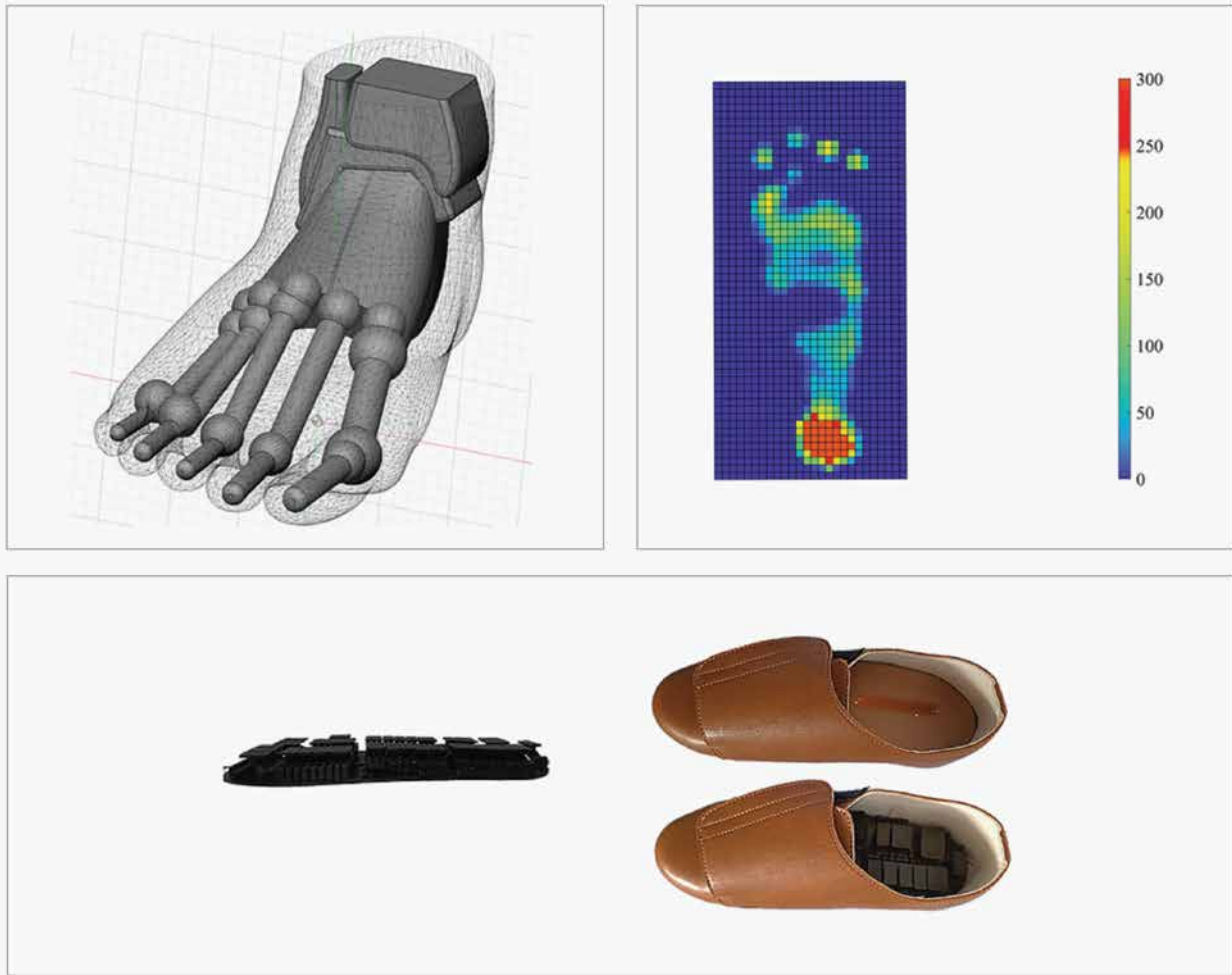
Clockwise from top: Simplified parameterised model of foot, plantar pressure obtained with digital twin of the foot, and insoles developed for diabetics
